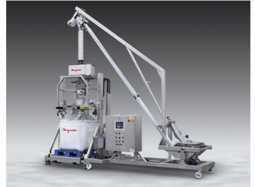
Mobile, Sanitary Bulk Bag Filling System from Flexicon is comprised of a TWIN-CENTERPOST™ Bulk Bag Filler with metal detection/removal, and a Tilt Down Flexible Screw Conveyor with clog-free dust-containment system. Programmable controls automate all filling and conveying functions.
