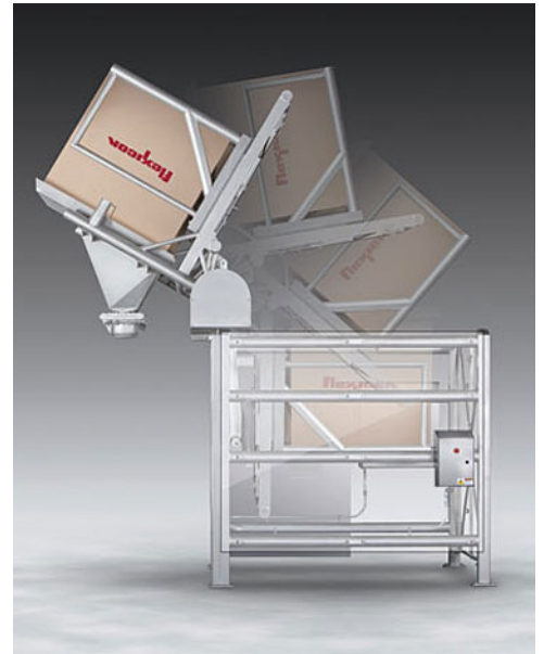
TIP-TITE® Sanitary Box Dumper forms a gasketed, dust-tight connection between the container and the equipment, tips the container to 45, 60, or 90 degrees past horizontal, and discharges bulk material through a slide gate at controlled rates.
