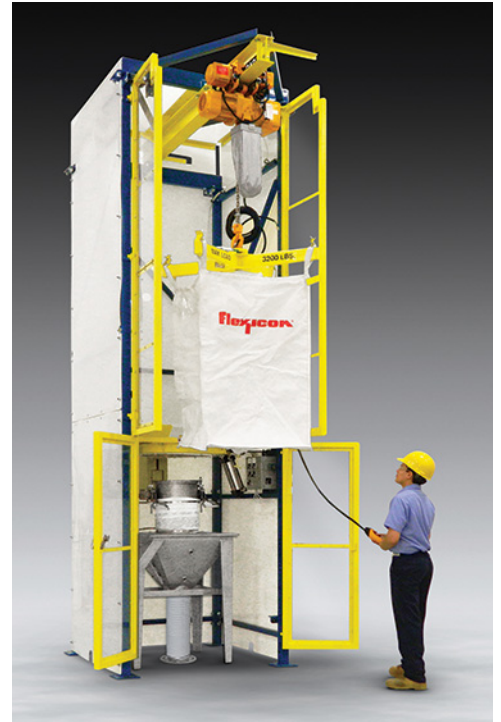
Flexicon BULK-OUT® BFC Discharger with five-sided enclosure vented to a plant's dust collection system captures airborne dust escaping through the seams or fabric of bulk bags.
