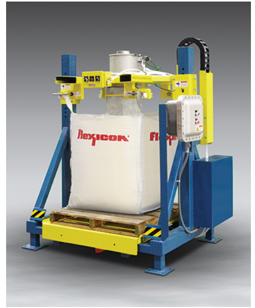
Flexicon low profile TWIN-CENTERPOST™ Bulk Bag Filler has XP controls for deaeration deck.
