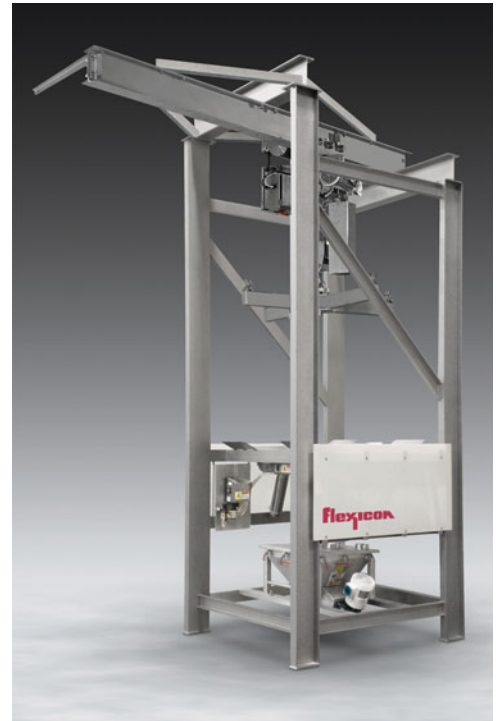
Open-channel stainless steel construction of Flexicon Bulk Bag Discharger eliminates internal voids where contamination can breed, and allows rapid sanitizing and inspection.
