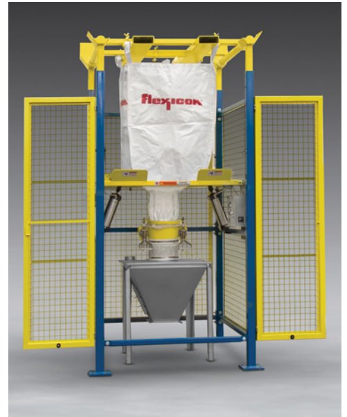
Steel safety enclosure of BULK-OUT® Model BFF Bulk Bag Discharger ceases operation of moving parts when safety interlocked doors are open.
