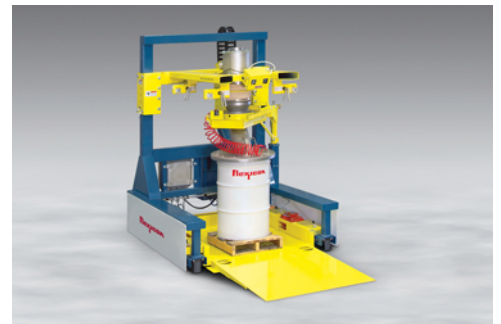
In drum-filling mode, the feed chute can fill one drum (shown) by weight, or multiple drums by automatically indexing to successive drums after each is filled.
