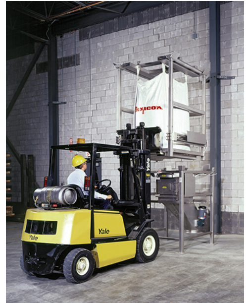
Split Frame Unloader allows discharging of bulk bags and rigid totes from mezzanines and other low headroom areas. The flanged discharge chute of the frame shown is offset to direct material into an off-center receiving vessel below a mezzanine.
