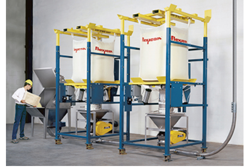
Major ingredients sourced from bulk bags are weighed automatically while minor, pre-weighed ingredients are dumped manually.
