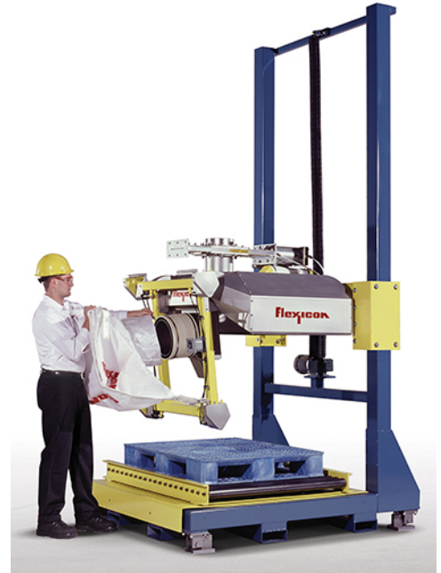
Design precludes stepping on roller conveyors and reaching into fill head
