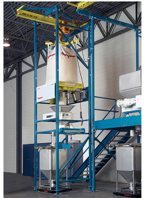
Bulk-Bag-to-Bin Weigh Batching System discharges material from bulk bags, de-lumps the product, and feeds it gravimetrically into rigid bins placed on a floor scale that is linked to a PLC.
