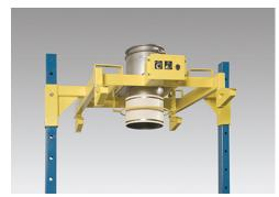
Flexicon's lowest cost bulk bag filler is a lighter duty version of the company's patented TWIN-CENTERPOST™ design offering extreme structural integrity and easy access to bag connection points at minimum cost.
