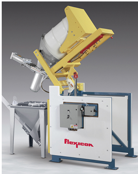
TIP-TITE® Drum Dumper seals drum rim against a discharge cone, tips the drum, mates the cone against a gasketed connection, and discharges bulk material dust-free through a slide gate valve.
