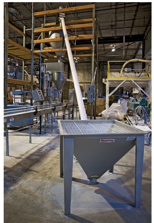
Blended perlite mixture discharges from bulk bag into the 8 cu ft (0.23 cu m) capacity stainless steel hopper (top), as the 30 ft (9.1 m) long flexible screw conveyor moves the material to the surge hopper above the packaging machine (above).
