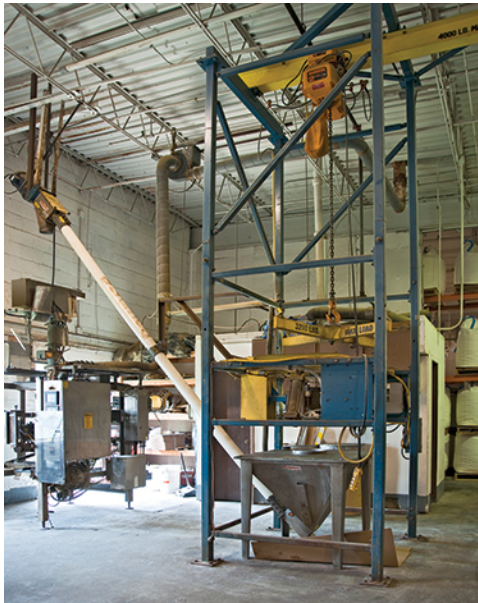
APCO Packaging employs bulk bag dischargers and flexible screw conveyors in repackaging various industrial, household and personal care products. This BULK-OUT® BFC discharger from Flexicon features a cantilevered I-beam with electric hoist and trolley.
