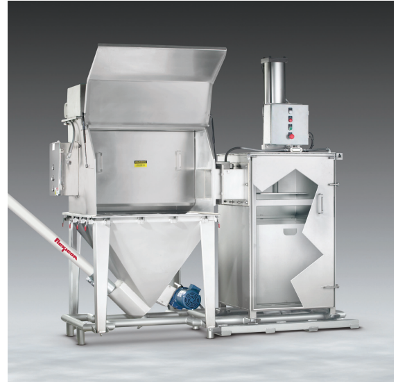
Self-contained Bag Dump System with dust collector, flexible screw conveyor and bag compactor, streamlines installation and allows easy relocation. The entire airtight system is under negative pressure, containing dust when bags are dumped, as well as when empty bags are pushed through the chute and compacted.
