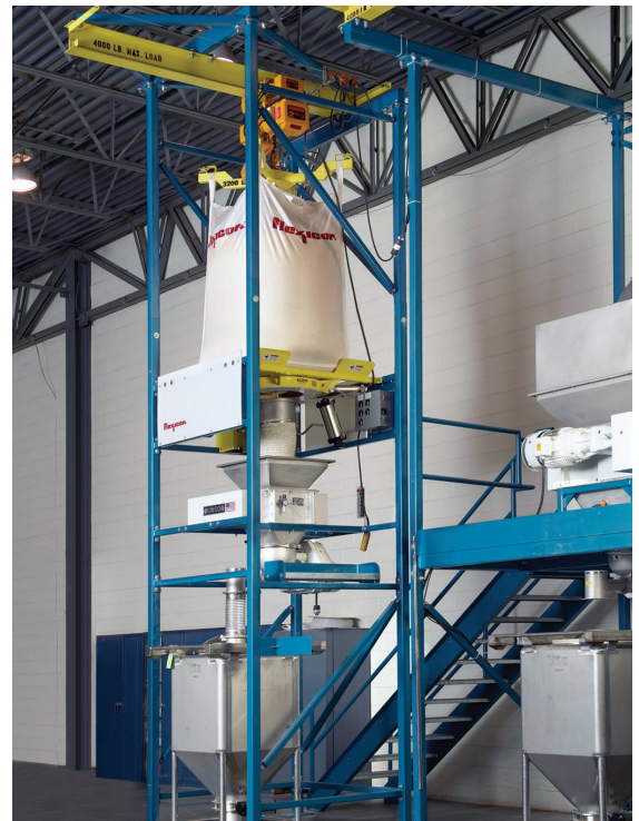
Bulk-Bag-to-Bin Weigh Batching System discharges material from bulk bags, de-lumps the product, and feeds it gravimetrically into rigid bins placed on a floor scale that is linked to a PLC.
