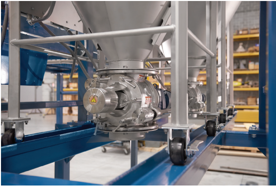
Caster-mounted, the cone hoppers can be rolled in C-channels to either side of the central filling position for cleaning offline, while another hopper is in use.
