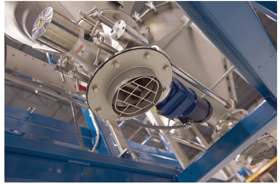
Hoppers discharge through stainless steel rotary valves equipped with support rails that allow the rotor assembly to separate from the valve body without tools for rapid sanitizing.
