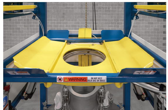
Two types of FLOW-FLEXER® pneumatically actuated devices are employed to promote complete discharge: one with rams that press opposing sides of the bag, and the other with contoured plates that raise opposing bottom sides of the bag.
