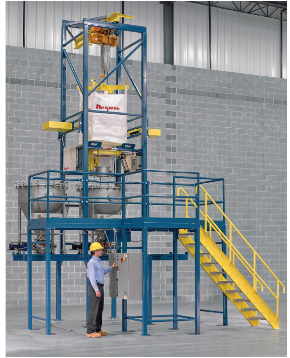
The hopper shuttle system of this BULK-OUT® Bulk Bag Discharging Station allows an emptied hopper to be rolled outside of the central filling position for cleaning and drying offline, while a second hopper is receiving material from a bulk bag and/or metering it into process equipment below the mezzanine.
