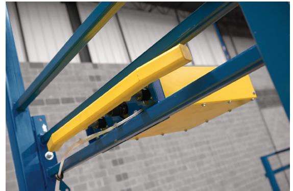
The hopper shuttle system of this BULK-OUT® Bulk Bag Discharging Station allows an emptied hopper to be rolled outside of the central filling position for cleaning and drying offline, while a second hopper is receiving material from a bulk bag and/or metering it into process equipment below the mezzanine.
