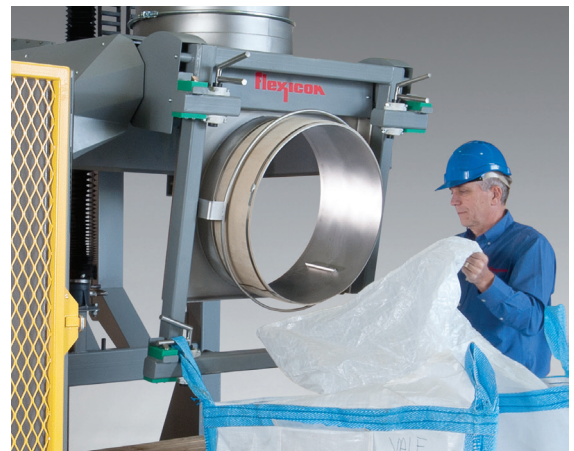
SWING-DOWN® Fill Head with wide-diameter spout seal allows safe, rapid connection of wide diameter bag spouts for passage of filter cake, aggregates, metal powders, abrasive minerals, dry chemical additives and irregular bulk materials.
