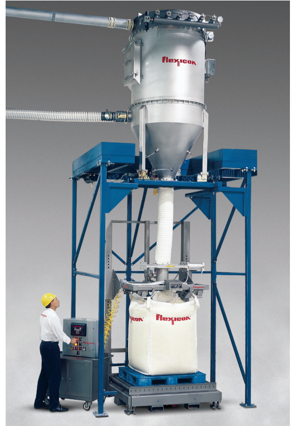
The filter receiver's load cells transmit weight gain information to the system controller that stops the conveyor once a pre-selected batch weight, equivalent to that of one full bulk bag, has been accumulated.
