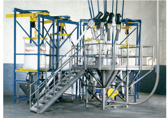
Feeds and weighs ingredients, and transports pre-weighed batches
