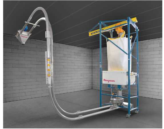
The automated Bulk Bag Weigh Batching System from Flexicon meters ingredients from a Bulk Bag Discharger into a FLEXI-DISC® Tubular Cable Conveyor that transports batches of a specified weight to a downstream process.
