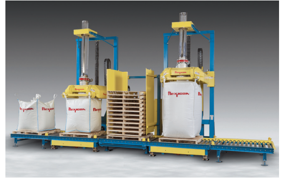
Automated roller conveyor with photoelectric eyes moves pallets directly under Swing-Down fill heads that allow connection of bag loops and spouts safely and rapidly at floor level.
