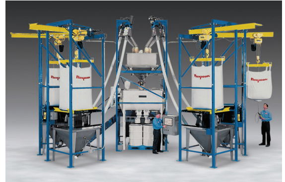
Automated system is comprised of four bulk bag unloaders equipped with flexible screw conveyors, a central gain-in-weight hopper and a ribbon blender that discharges into shipping containers.
