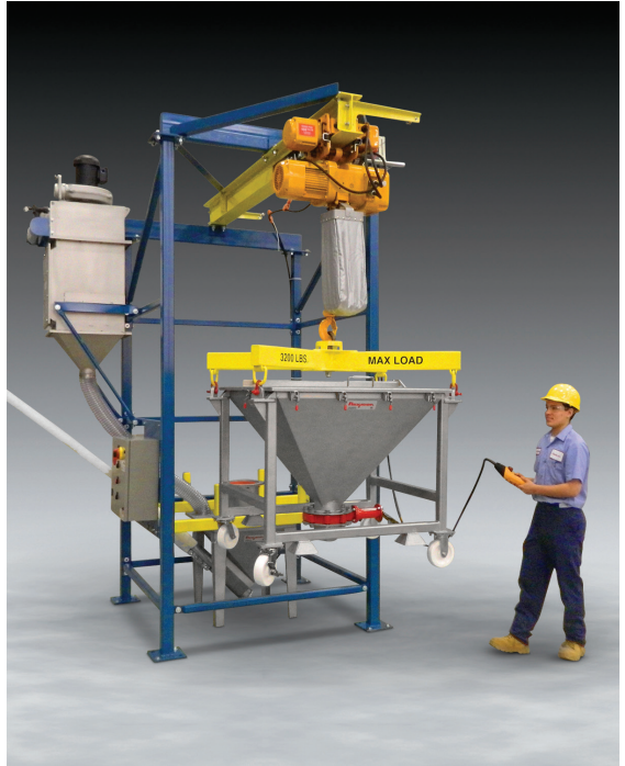
Flexicon's IBC Discharger raises and positions rigid Intermediate Bulk Containers without the use of a forklift, makes a dust-tight connection to a surge hopper available with outlets to charge a flexible screw conveyor (shown), tubular cable conveyor or pneumatic conveying system.
