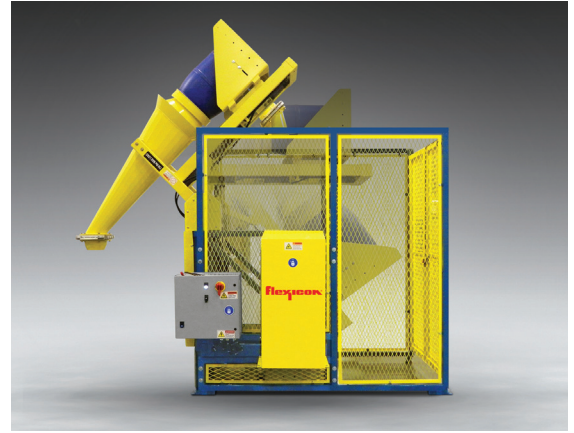
TIP-TITE® Drum Dumper with elongated discharge cone seals the drum rim before tipping the drum, seating the spout of the discharge cone against a gasketed receiving ring on vessel lids for dust-free discharging.
