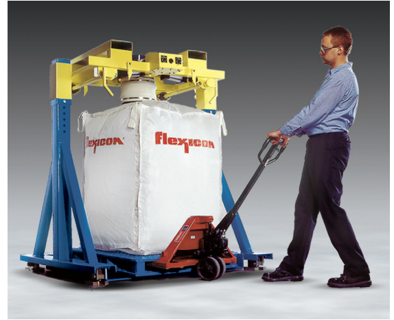
Flexicon's Low Profile Bulk Bag Filler allows removal of loaded bags using a pallet jack, eliminating the need for a forklift.
