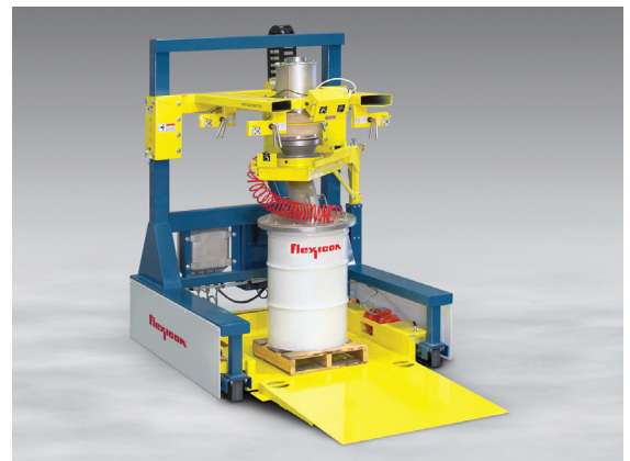
In drum-filling mode, the feed chute can fill one drum (shown) by weight, or multiple drums by automatically indexing to successive drums after each is filled.
