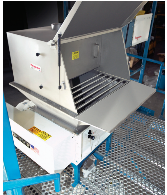
Manual Dumping Station draws airborne dust from the operator's atmosphere during dumping from bags, boxes, drums and other containers.
