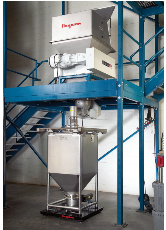
Manual Dump to Rigid Bin Weigh Batching System eliminates dust during manual dumping activities, de-lumps the material, and feeds it gravimetrically into rigid bins placed on a floor scale.
