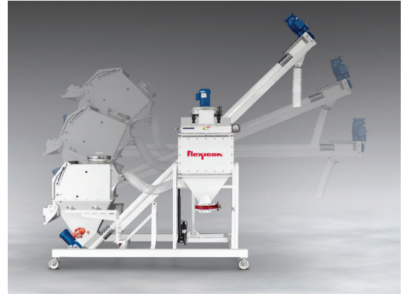
Mobile Tilt Down Flexible Screw Conveyor System with multi-purpose hood and integral dust collector allows manual dumping from handheld sacks, discharging from bulk bags, and transferring of material to elevated downstream equipment, dust-free.
