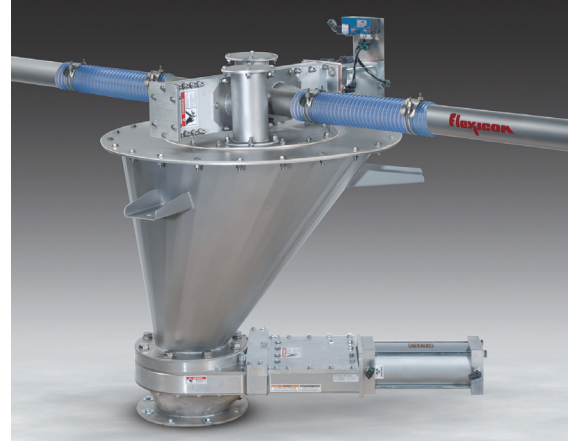
Fill/Pass Valve of Flexicon's pneumatic weigh hopper allows material to pass through the valve or to fill a hopper based on weight gain signals transmitted from load cells to the system's controller.
