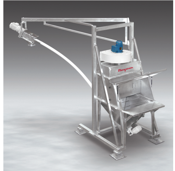
An integral flexible screw conveyor is supported by a boom that cantilevers from the frame of the system which is supported on load cells, allowing loss-of-weight batching directly from paper sacks and other manually dumped containers.
