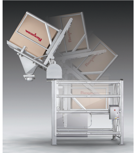
TIP-TITE® Sanitary Box Dumper forms a gasketted, dust-tight connection between the container and the equipment, tips the container to 45, 60, or 90 degrees past horizontal, and discharges bulk material through a slide gate at controlled rates.
