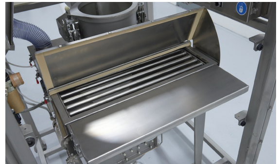
Manual dumping station of BULK-OUT® Bulk Bag Weigh Batch Unloading System shown with hinged hopper lid and bag tray in raised positions, ready to receive minor ingredients dumped manually.
