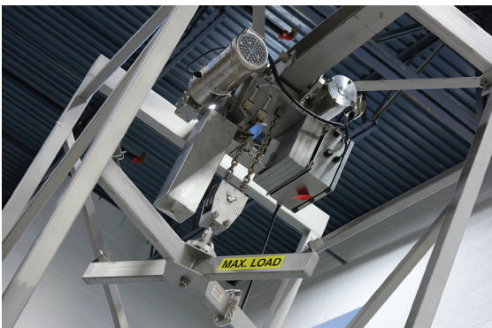
The all-stainless-steel flexible screw conveyor discharge, complete with motor drive, air purged packing gland for the drive shaft and pneumatically-actuated slide gate valve, is rated for wash down.
