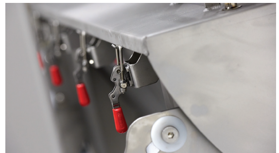
Stainless steel over-center quick-release clamps secure the hinged hopper lid during discharge of material from bulk bags.
