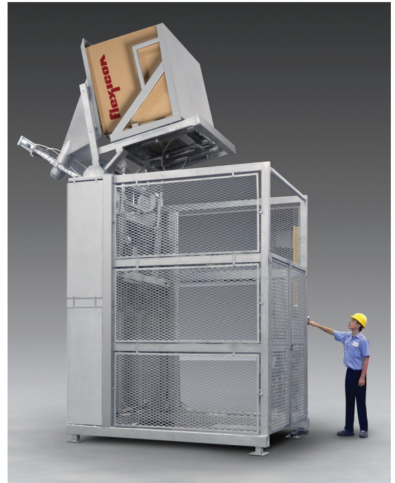
Container platform of sanitary TIP-TITE® High-Lift Box/Container Dumper raises to form dust-tight seal between container and discharge hood before the assembly is raised vertically and then tipped, mating the hood outlet with the gasketed inlet port on any receiving vessel 6 to 10 ft (1830 to 3050 mm ) high.
