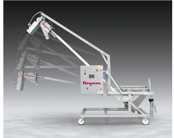
Flexicon's Mobile Sanitary Flexible Screw Conveyor can be tilted down to clear doorways 7 ft (2134 mm) in height, and rolled through aisles as narrow as 42 in. (1067 mm).
