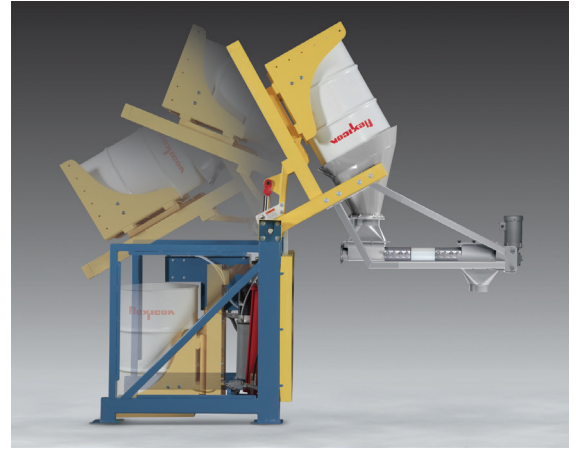
Self-contained Drum Dump Feeder discharges bulk material from drums and feeds it volumetrically to downstream equipment. Cantilevered flexible screw conveyors are offered in custom lengths oriented horizontally (shown), or at an incline, for the purpose of elevating as well as metering the material.
