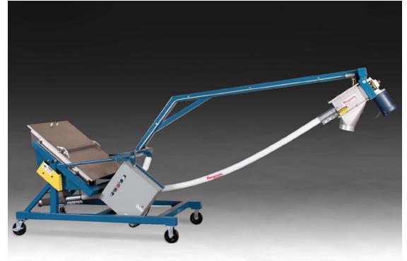
Bulk conveyor shown with hopper, support boom and conveyor assembly tilted down, allowing the unit to pass through narrow aisles, around corners and under obstructions. Horizontal orientation of conveyor tube's bottom end allows flexible screw to be removed easily for thorough cleaning and inspection.
