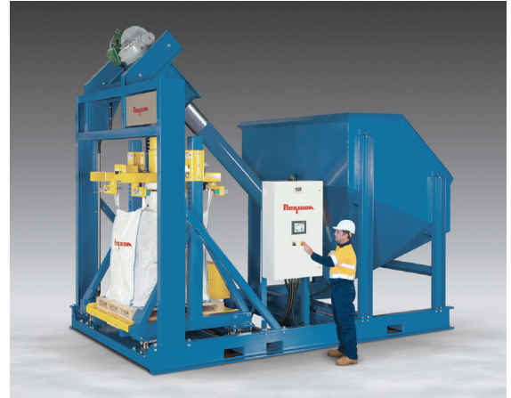
Ultra-heavy-duty, skid-mounted bulk bag filling system includes a patented TWIN-CENTERPOST™ frame, flexible screw conveyor, high capacity hopper, and PLC to control automated filling functions.
