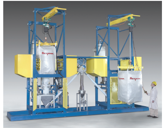
Bulk Bag Weigh Batch Eductor System features dual bulk bag unloaders, each with integral bulk bag conditioners and flexible screw conveyors feeding a central eductor that feeds solid material into a liquid stream.
