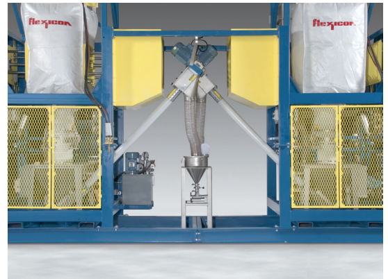
Flexible screw conveyors gravimetrically feed bulk solids into a central solid-liquid eductor that blends the material into a liquid stream in ratios set by the user.
