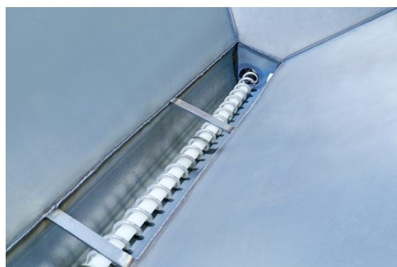
The hopper's bottom features a U-shaped channel that exposes the flexible screw for the entire length of the vessel, allowing material entering the hopper at any point to charge the conveyor.
