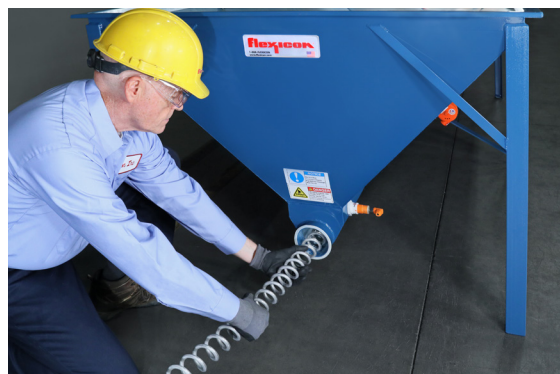
Quick-disconnect clamps near the drive point and a removable cleanout cap at the opposite end of the conveyor (shown) allow for easy removal and cleanout of the flexible screw during material changeovers.
