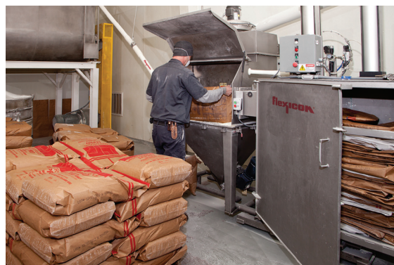
By blending in-house, Franklin Farms East can meet increased demand and expand its product line. The flexible screw conveyor transports minor ingredients being emptied at the bag dump station to the blender in background.
