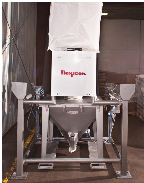
Limited headroom requires a forklift to suspend bulk bags above the lower half of this split-frame BULK-OUT® bulk bag discharger. Once the room is enlarged with a higher ceiling, bulk bags will be loaded at floor level into the top half of the split-frame, which will then be forklifted with bag intact, onto the lower half of the frame, within inches/centimeters of the ceiling.
