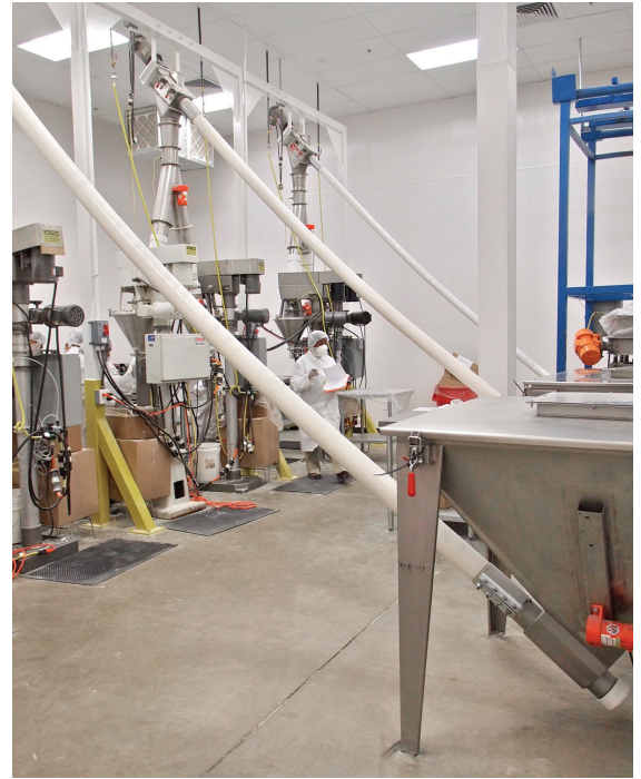
Powders remain totally enclosed from bulk bags to packaging machines, improving plant cleanliness.
