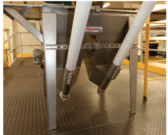
Two types of cocoa powder are emptied into the twin hopper while dust is removed by vacuum. The two flexible screw conveyors move each powder, alternately, to the mixer.
