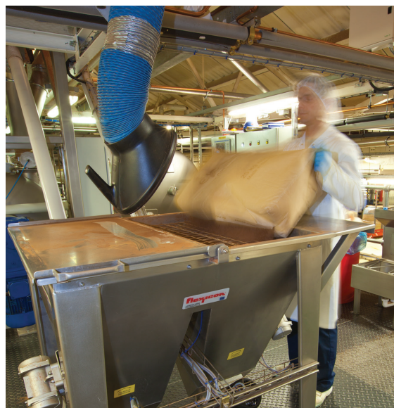
Two cocoa powders are transferred from the twin hopper through each flexible screw conveyor to the mixer, while sugar enters the mixer from pneumatic receiving hoppers above. The entire batching/blending process is controlled by PLC.
