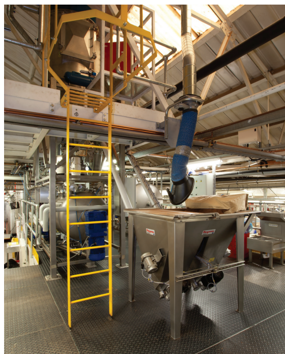
Two cocoa powders are transferred from the twin hopper through each flexible screw conveyor to the mixer, while sugar enters the mixer from pneumatic receiving hoppers above. The entire batching/blending process is controlled by PLC.
