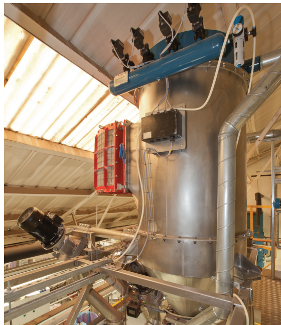
Sugar is fed into the mixer below from the 550 kg pneumatic receiving hopper. At left, cocoa powder enters the mixer through the discharge end of the flexible screw conveyor and downsput.
