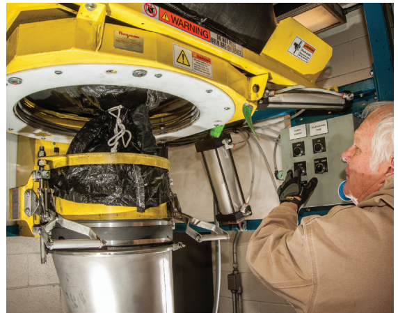
Operator pulls bag spout through the POWER-CINCHER® control valve, and then onto the SPOUT-LOCK® clamp ring that is raised by a pneumatically powered TELE-TUBE® telescoping tube.
