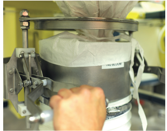
Once a bag is hoisted into position, an operator pulls the bag spout over a SPOUT-LOCK® clamp ring, which creates a secure, dust-tight connection between the clean side of the bag spout and the clean side of a TELE-TUBE® telescoping tube, which maintains constant downward tension to promote complete discharge.
