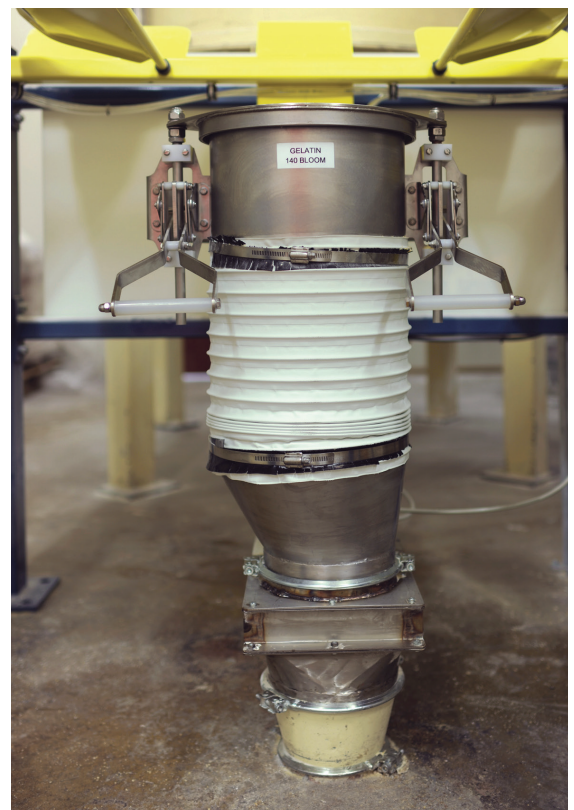
Ingredients such as milk, powder, sugar, starch, and sour coating powder arrive in 1.1 tonne bulk bags, and are gravity fed into the processing lines where feasible.
