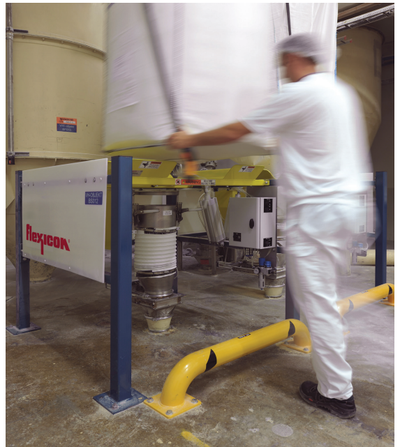
Nidar AS added twin bulk bag dischargers from Flexicon to handle two types of starch in a tight space on the plant's fourth floor.
