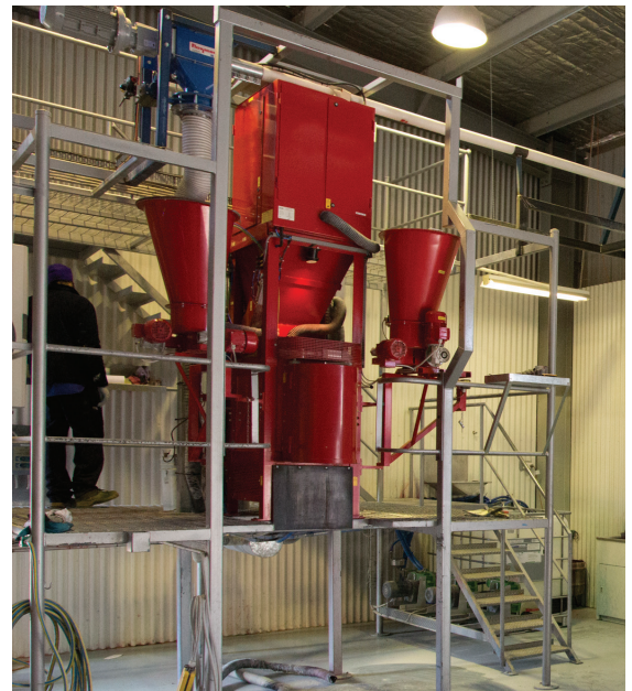
Iris valve prevents uncontrolled bursts of material and dust when bag spout is untied.
