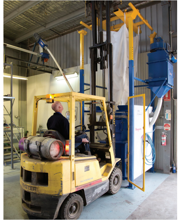
Forklift loads a bulk bag onto the discharger frame, which is fitted with dust collector (right).
