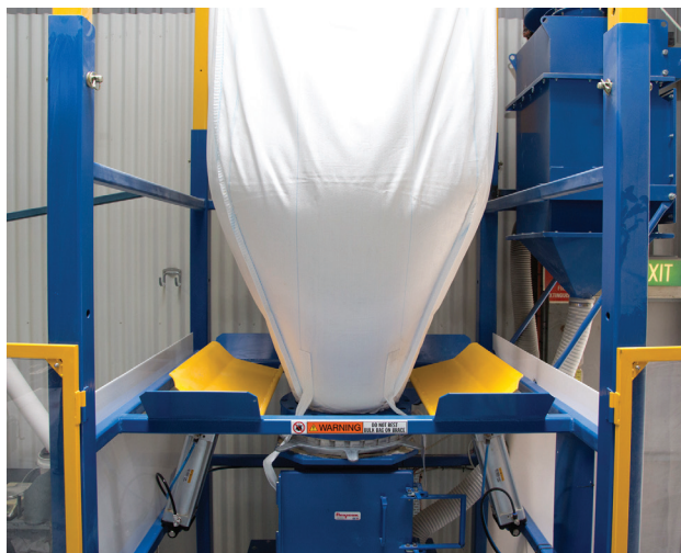
FLOW-FLEXER® plates raise and lower the bag to promote complete evacuation.
