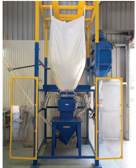
Iris valve prevents uncontrolled bursts of material and dust when bag spout is untied.
