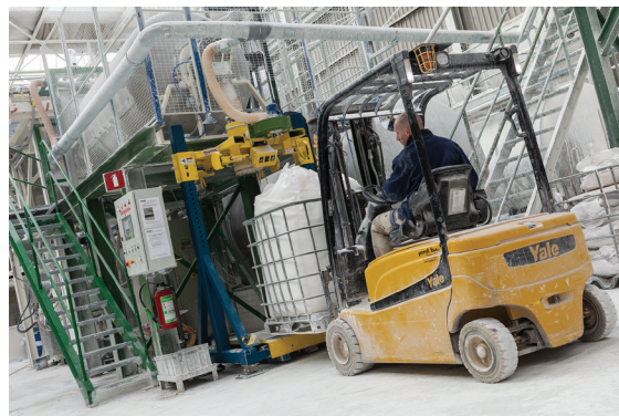
Forklift truck removes palletised filled bag.
