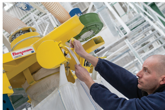
The operator slides the bag spout onto the inflatable collar and attaches bag straps to retractable hooks that support the bag during filling.
