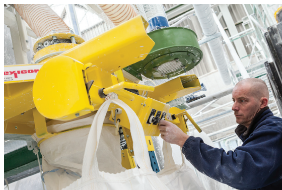
Operator activates the inflatable collar to form a secure, dust-tight connection, and then actuates the bag inflation blower to remove creases in the bag prior to filling.
