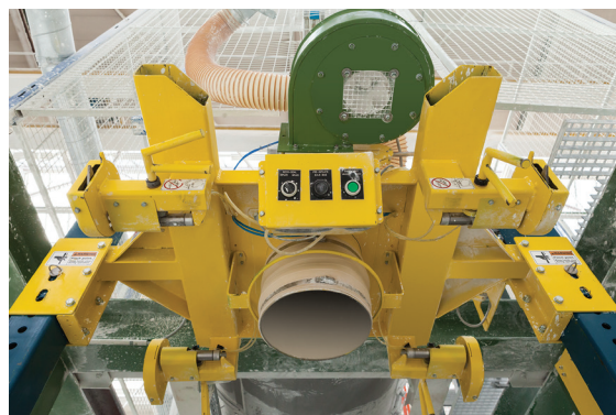
View from below shows the fill head, forklift sleeves for adjusting the fill head height, retractable bag hooks for supporting the bag, and vent for capturing displaced air and dust.
