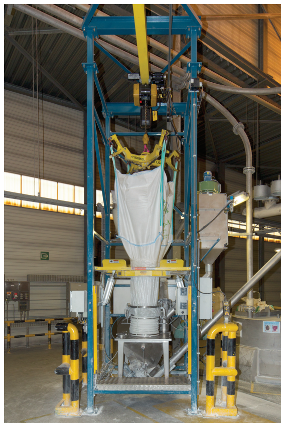
Flexicon bulk bag discharger positions the bag from a cantilevered I-beam with electric hoist and trolley and cross-shaped bag-lifting frame. The discharger provides complete evacuation of the bag, flow and dust control at the bag spout interface, and PLC control for automatic operation. The flexible screw conveyor transports talc to the blending hopper.
