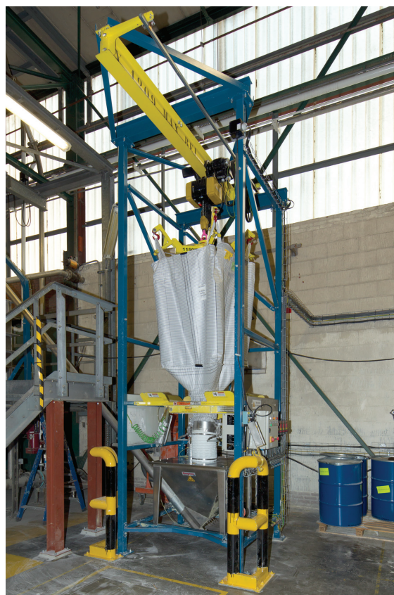
Automated, safe, and dust-free, the Flexicon discharger is equipped with an integral flexible screw conveyor that delivers impact modifier to the blending hopper.
