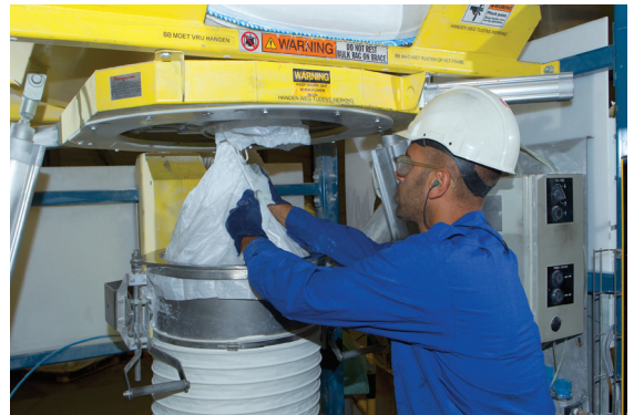
Operator pulls the bag's outlet spout through a POWER-CINCHER® flow-control valve, which prevents product leakage. He then connects the spout to a SPOUT-LOCK® clamp ring, which is mounted atop a TELE-TUBE® telescoping tube that promotes material flow and eliminates dust.
