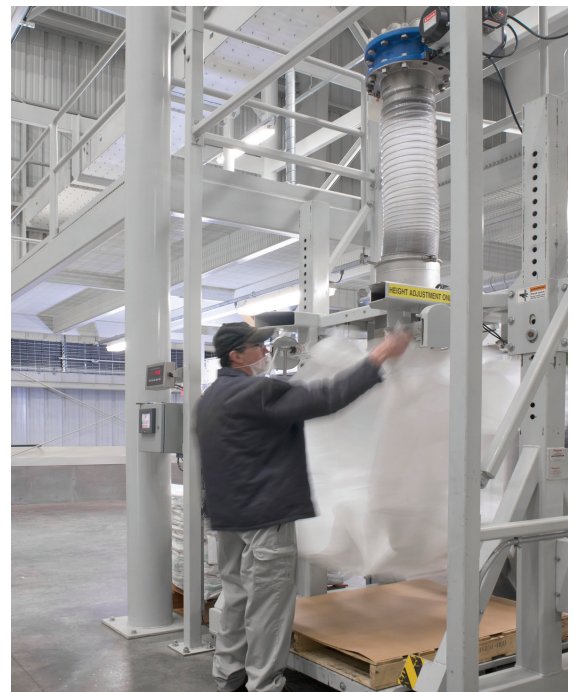
Tronox Western Australia semiautomatically fills and ships bulk bags of rutile (titanium dioxide) and zircon (zirconium silicate), which are mined and processed from native mineral sands.
