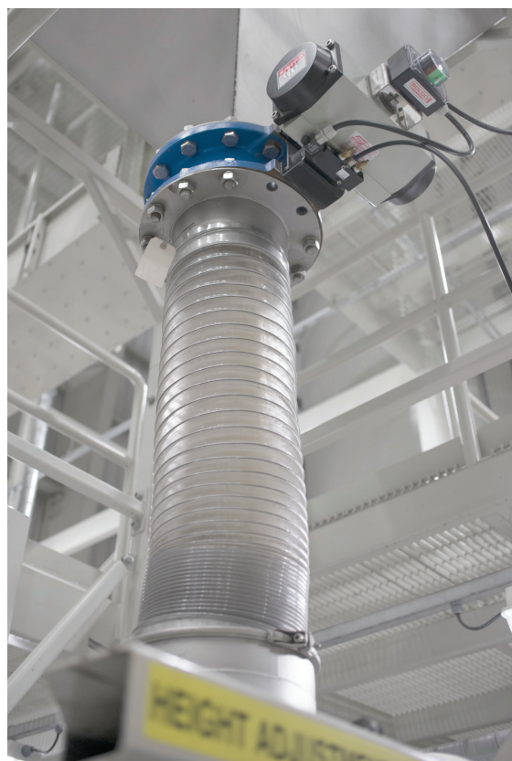
Rice descends from the hopper, through a dome valve and downspouting into the TWIN-CENTERPOST™ bulk bag filler.
