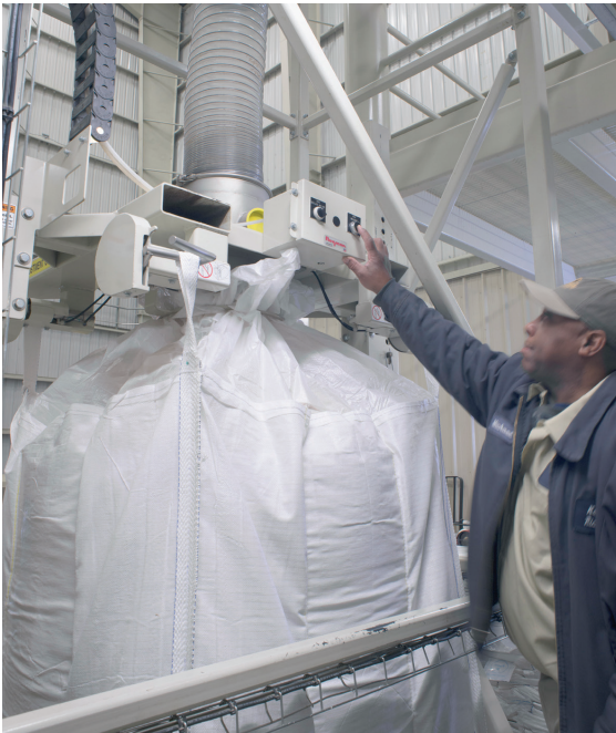
Operator inflates the bag, removing creases prior to filling.
