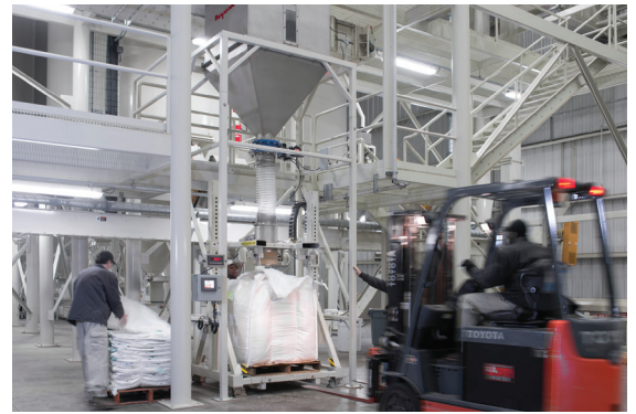
Forklift removes filled bag on pallet as operator readies another bag to be filled.
