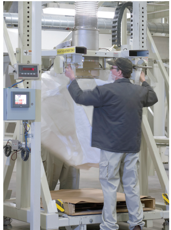
The special heavy-duty bulk bag filler doubles output per operator over former manual methods, and improves health and safety as filling is enclosed and dust-free.
