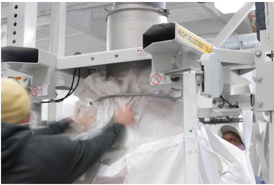
Bag spout is pulled over an inflatable collar which, together with a filtered air displacement vent, assure dust-free filling.
