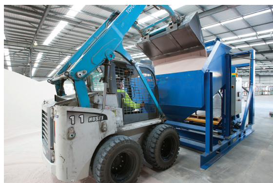
The 88 cu ft (2.5 cu m) capacity hopper can hold 7-8 tons (6.4-7.3 mt) of zircon or 5-6 tons (4.5-5.4 mt) of rutile.
