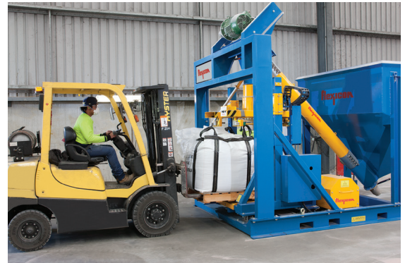
The special heavy-duty bulk bag filler doubles output per operator over former manual methods, and improves health and safety as filling is enclosed and dust-free.
