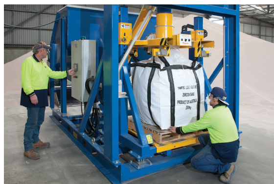
One operator attaches bag to the fill head as other operator pre-sets the bag weight and initiates filling at the PLC. The Twin-Centerpost design filler frame and heavy-duty outer frame impart strength for filling bags weighing between 2,200 to 4,400 lb (1,000 to 2,000 kg).
