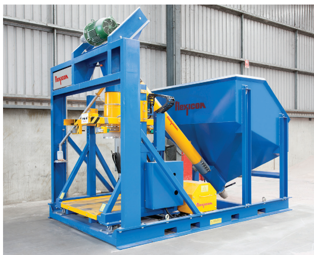
Skid-mounted mobile bulk bag filling station, nicknamed 'Rhonda' at the Tronox Henderson facility, consists of an 88 cu ft (2.5 cu m) capacity hopper, a 15 ft (4.5 m) long tubular screw conveyor, a Twin-Centerpost™ bulk bag filler, and PLC control.
